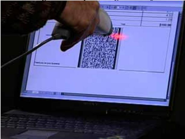
A 2D barcode is scanned directly from a computer's video display.
